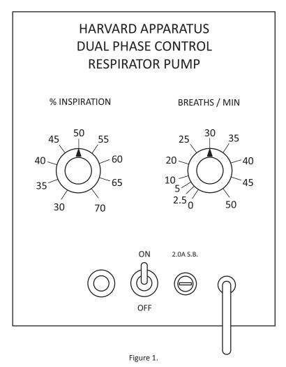
Control Panel for Large Animal Volume Controlled Ventilator, Model 613
